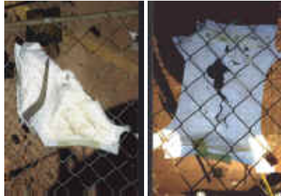
Photographs of a treated diaper exposed to the outside weather at one-week intervals
